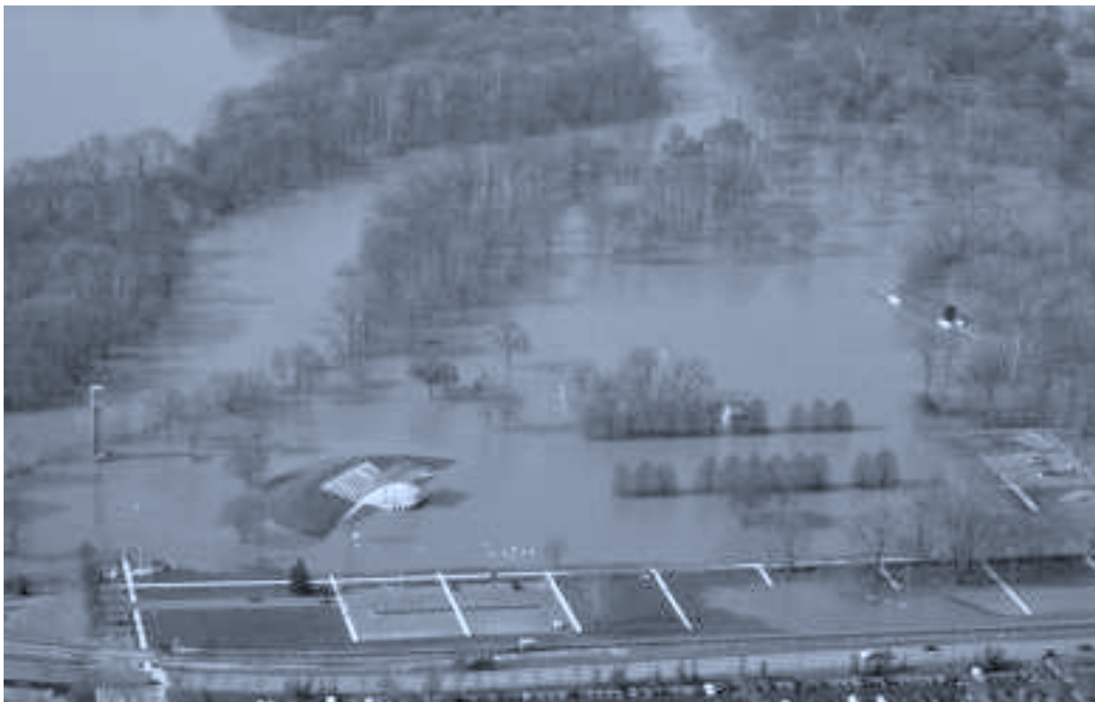
9. Aerial photograph during a flood, Mill Race Park, Columbus, Indiana, by Michael Van Valkenburgh Associates, 1989–93. The elevated plinth of the playground and the high masses of the amphitheater and lookout mound register the fluctuation of the river level and function as memory devices. (photo: courtesy of Michael Van Valkenburgh Associates)
