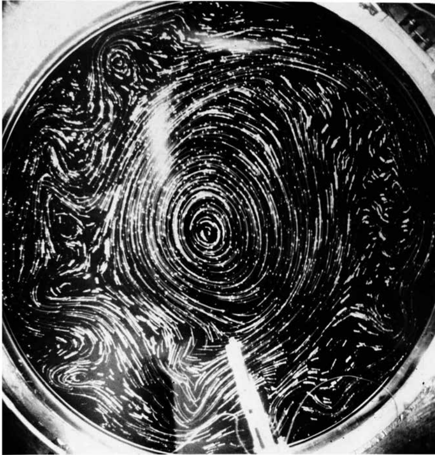
136. Convection in a rotating cylinder. The flow pattern in a rotating "dishpan" heated at the rim and cooled at the center bears a remarkable resemblance to the basic features of the middle-latitude atmosphere of the Earth. Here water 4 cm deep in a cylinder 19.5 cm in diameter is rotating counterclockwise at 30 revolutions per second,
