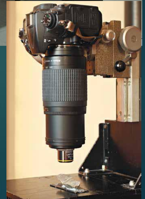
Long working distance Olympus LMPlanFL 10x/0.25 microscope objective coupled to a 70–300 mm telephoto zoom lens. Cliché H Plisson
